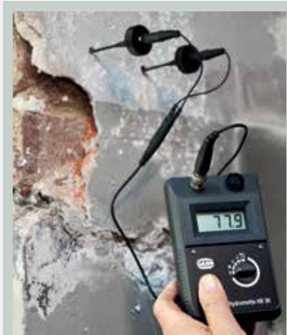
APPLICATION HB 30 together with an M 25-100 brush electrode pair
